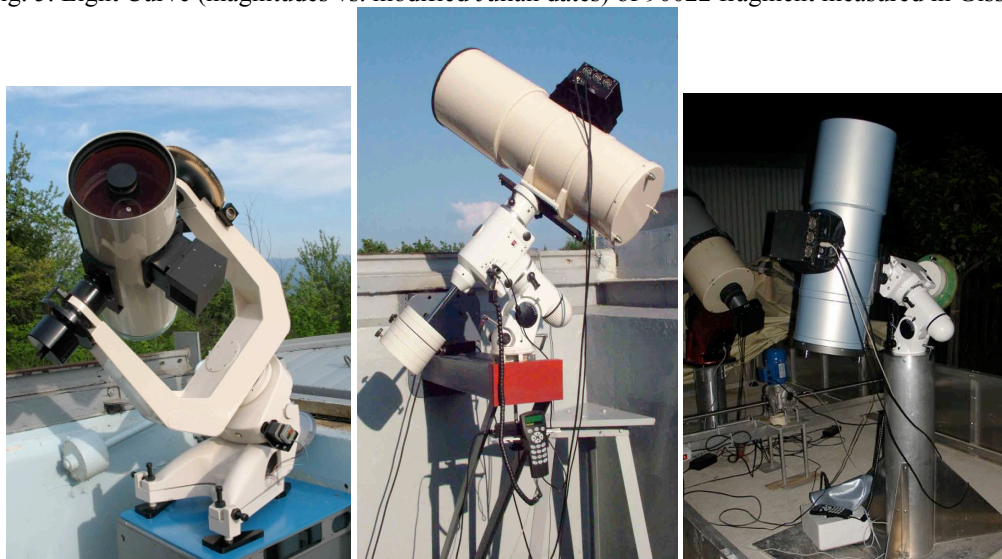
Fig. 6. 22 cm survey telescopes with FOV of 4°: PH-1 in Nauchny, ORI-22 in Ussuriysk, ORI-22 in Colleparado.
