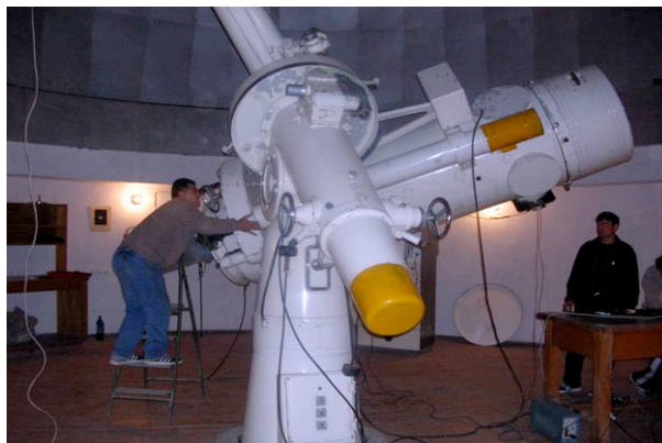
Fig. 4. Refurbished 70 cm telescopes for faint fragments: AZT-8 in Gissar and AS-32 in Abastumani.
