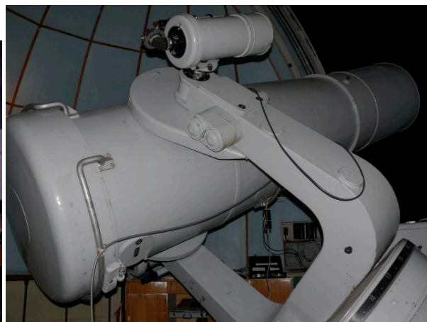
Fig. 4. Refurbished 70 cm telescopes for faint fragments: AZT-8 in Gissar and AS-32 in Abastumani.
