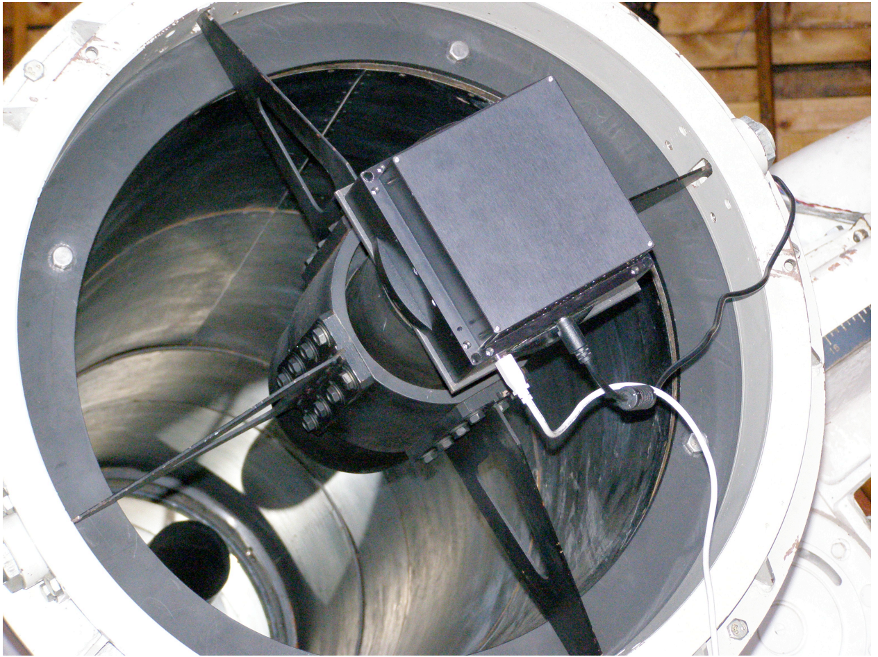
Fig. 1 The prime focus corrector and CCD established at the top of AZT 14 telescope.
